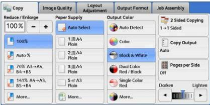
Press [service home] button, select [Copy], select each tab, and configure features as necessary, then press [start]
