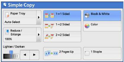
Press [service home] button, select [Simple Copy], select each tab, and configure features as necessary, then press [start].
